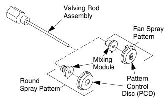
Fig. 3: Mixing Module & PCD
