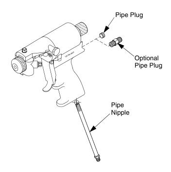
Fig. 9: Air Inlet Configuration
