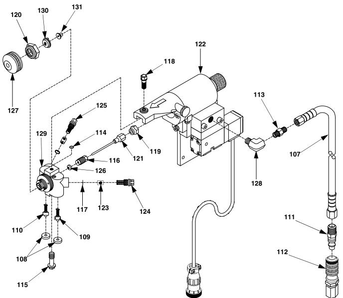
Fig. 21: GX-8P Spray Gun Final Assembly
