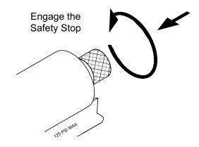
Fig. 4: Safety Stop - Engaged
