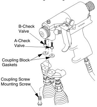
Fig. 8: Install Coupling Block
