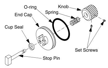
Fig. 17: End Cap/Safety Stop Assembly
