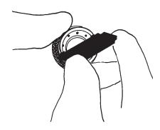
Fig. 19: Unthread Cap from PCD Body
