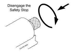
Fig. 5: Safety Stop - Disengaged
