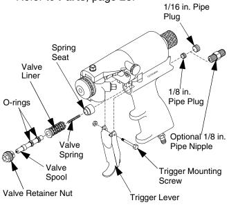
Fig. 18: Replace Trigger Valve O-Ring
