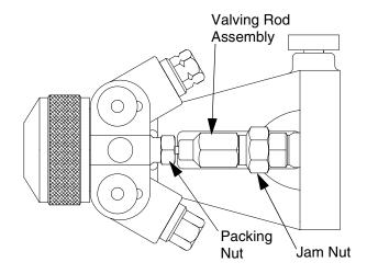
Fig. 10: Valving Rod Adjustments
