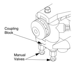
Fig. 7: Open Manual Valves
