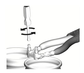
Fig. 13: Open Manual Valves
