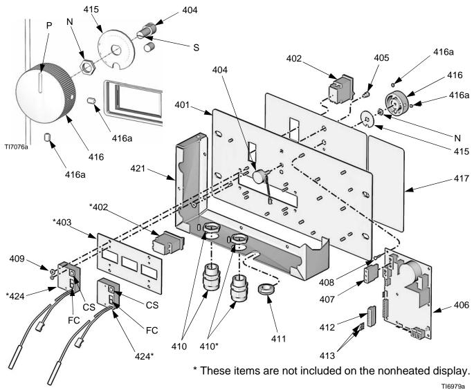
Fig. 11. Control Module (Heated Model Shown)
