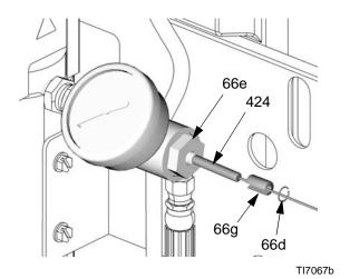
Fig. 10. Temperature Sensor
