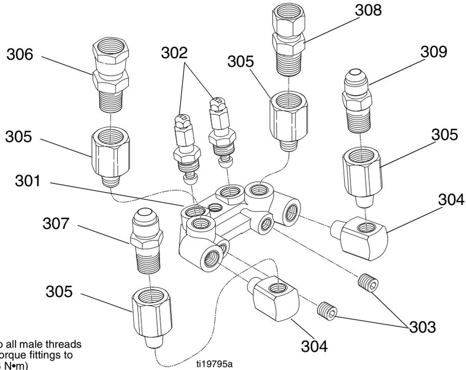
Apply pipe sealant to all male threads prior to assembly. Torque fittings to 120-130 in-lb (14-15 N•m)
