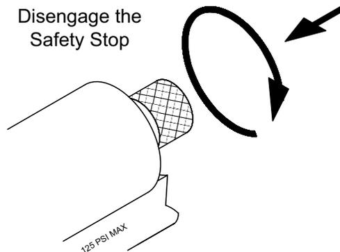
FIG. 5: Safety Stop - Disengaged
