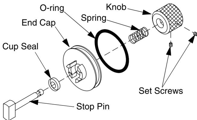
**FIG. 17: End Cap/Safety Stop Assembly**
