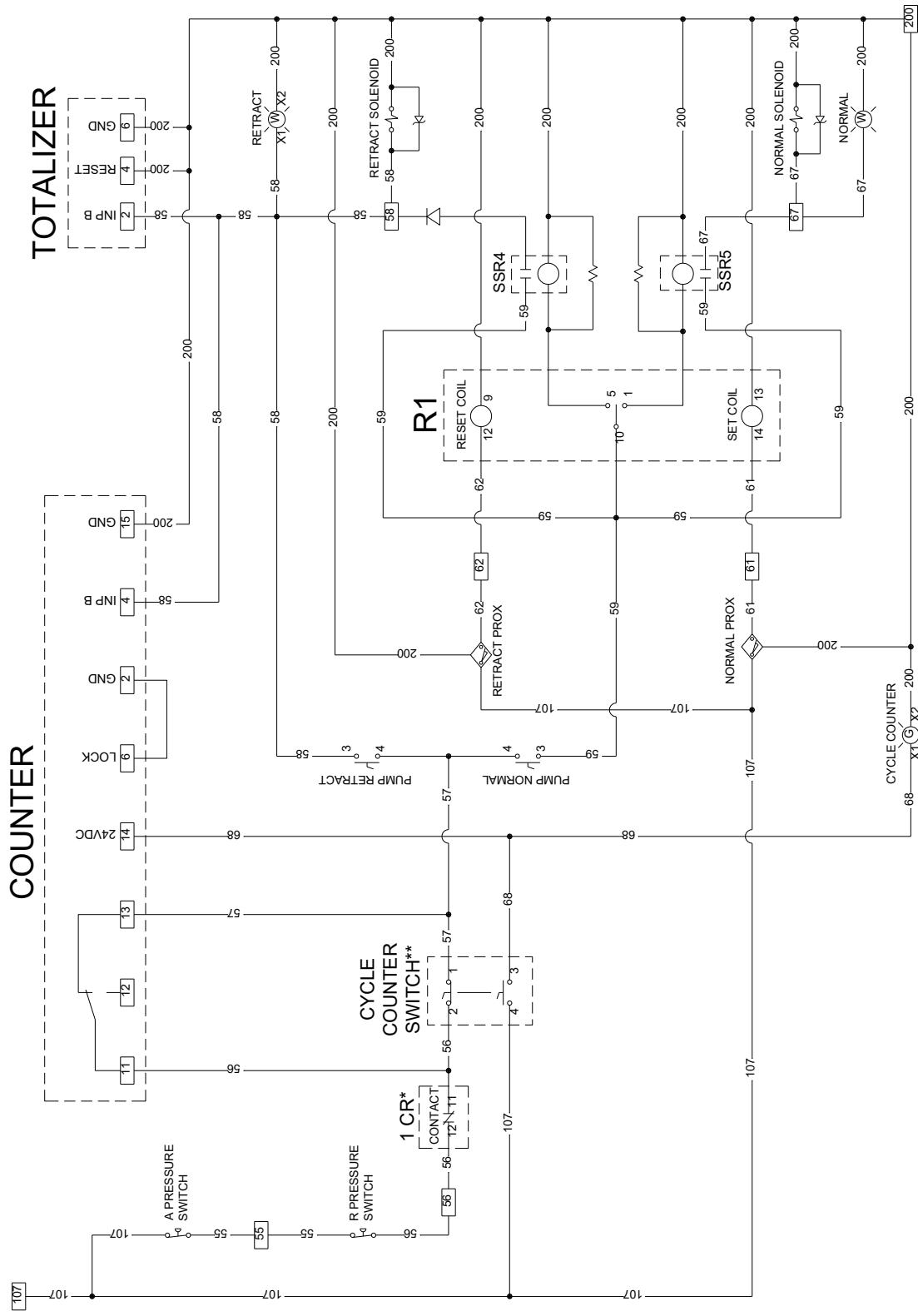
\*See Pressure Balance Control Circuit (Pg. 75) for complete 1 CR wire connections
