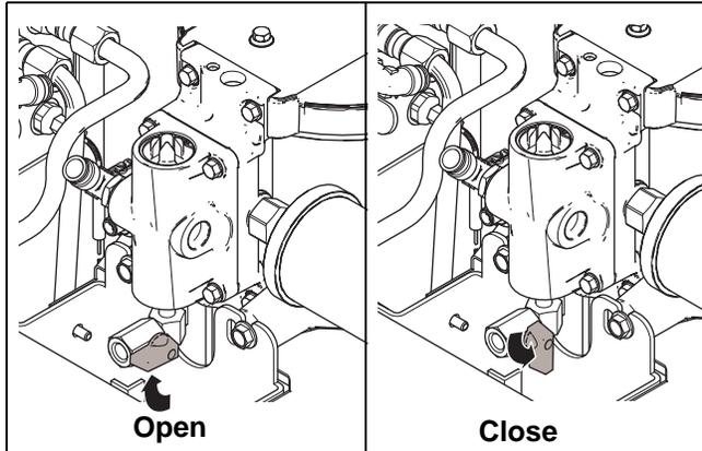
2. Trigger the gun until pumps stop at the bottom and relieve pressure.
