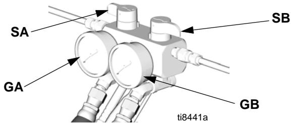
10. Check fluid pressure gauges (GA, GB) to ensure proper pressure balance. If imbalanced, reduce pressure of higher component by slightly turning PRESSURE RELIEF/SPRAY valve for that component toward PRESSURE RELIEF/CIRCULATION, until gauges show balanced pressures.
