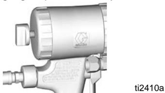
13. Test spray onto cardboard. Adjust the air regulator to get the minimum fluid pressure that results in a good spray pattern.
