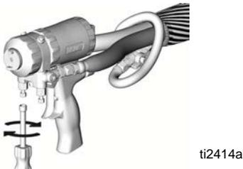
12. Disengage gun piston safety lock.
