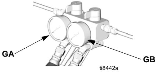
16. Open gun fluid manifold valves A and B.
