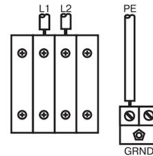
**200-240 V ac, 3-phase Delta:** Use a screwdriver to connect three power leads to top three left terminals as shown. Connect green to ground (GND). See page 18 for proper jumper positions.
