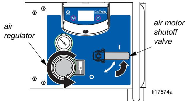
7. Open the air motor shutoff valve.
