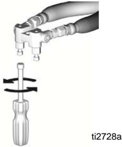
3. Attach gun fluid manifold. Connect gun air line. Open air line valve.
