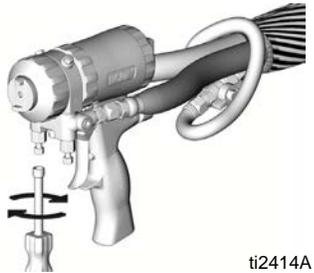
17. Disengage gun piston safety lock.
